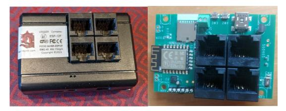
What does a LOGGER do? The LOGGER is a standalone IoT device that reads sensors and stores the data. The LOGGER captures 256 bytes of data on up to 128 sensors every few seconds. The data is stored on an SD card and kept permanently. About 20 years of data taken once every ten seconds fit on a 32Gb card.
